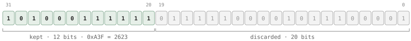
Figure 2 - the word 0xA3F7C2E1 at width 12: the kept bits read 101000111111, which is 0xA3F, group 2623.
